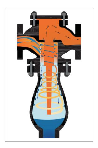
Separators can promote higher production for lower fuel cost because steam Contains more heat than hot water at the same pressure. Steam as dry as possible at point of use is important. Steam Separators improve the rate of heat transfer.
